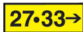
Outbound Destination Sign to Different Runways. More than one runway, separated by a dot, is shown where the taxiing route is common to both runways.
